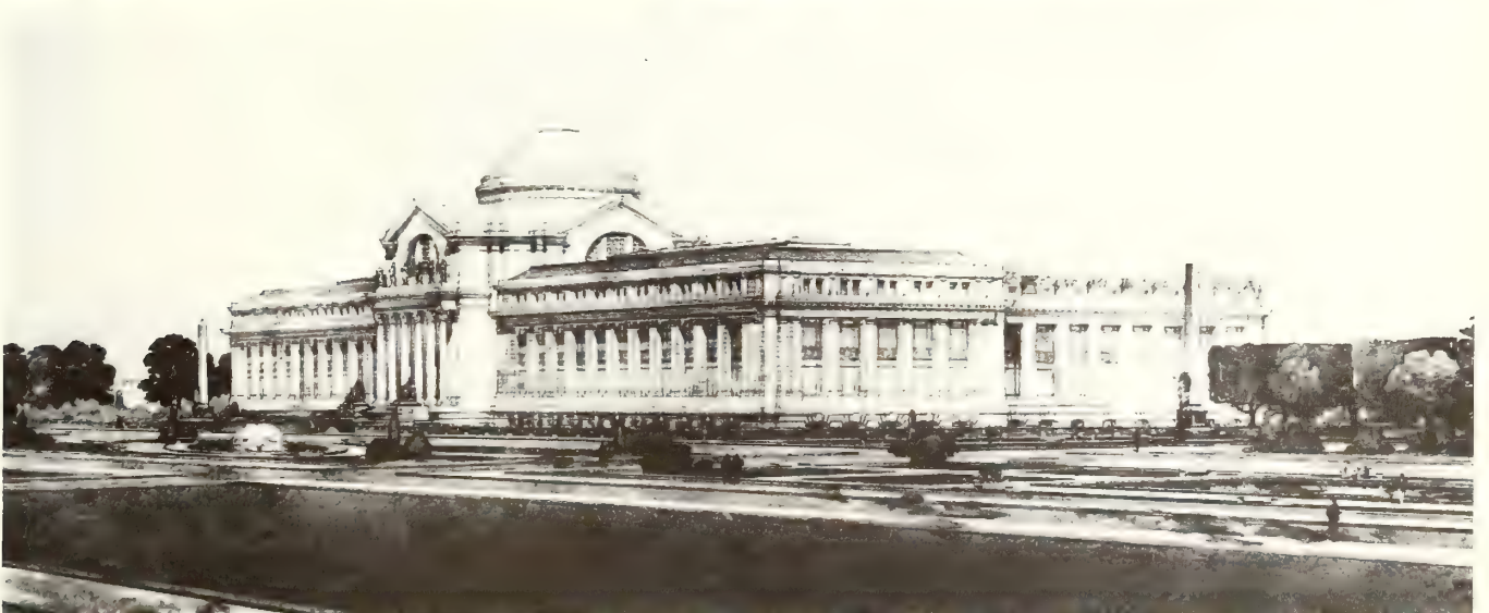
Three architectural sketches of the proposed New National Museum. Top, with a low mansard roof and a skylight around the central areas, as planned in July 1903. Middle, with the elaborate dome projected in 1904;
